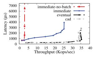
Fig. 6. Write-only workload: Latency vs. throughput. The figure plots the average latency against throughput by varying the number of clients for a write-only workload for different durability layers.
