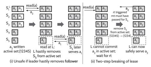
Fig. 5. Active set and leases. (i) shows how removing a follower hastily can expose non-monotonic states; (ii) shows how Orca breaks leases.
