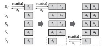
Fig. 4. Non-monotonic reads. The figure shows how non-monotonic states can be exposed atop CAD when reading at the followers.
